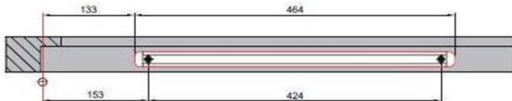
view of underside of transom
